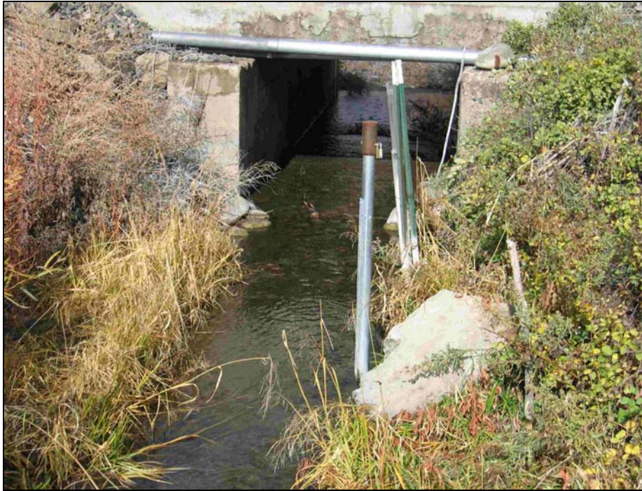
Figure 6. Locke Creek near mouth. October 28, 2005. The Aquarod® is housed in the metal pipe driven into the streambed.
