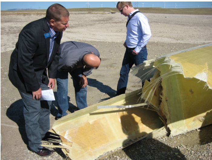
Senator Ed Buttrey examines a wind turbine that was struck by lightning.
