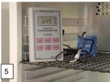
reading temperature measuring device to make process adjustments, place the wet bulb thermometer for easy access and readability, such as near a door or window (image 5). If immediate feedback is not a consideration (image 6), place the device
